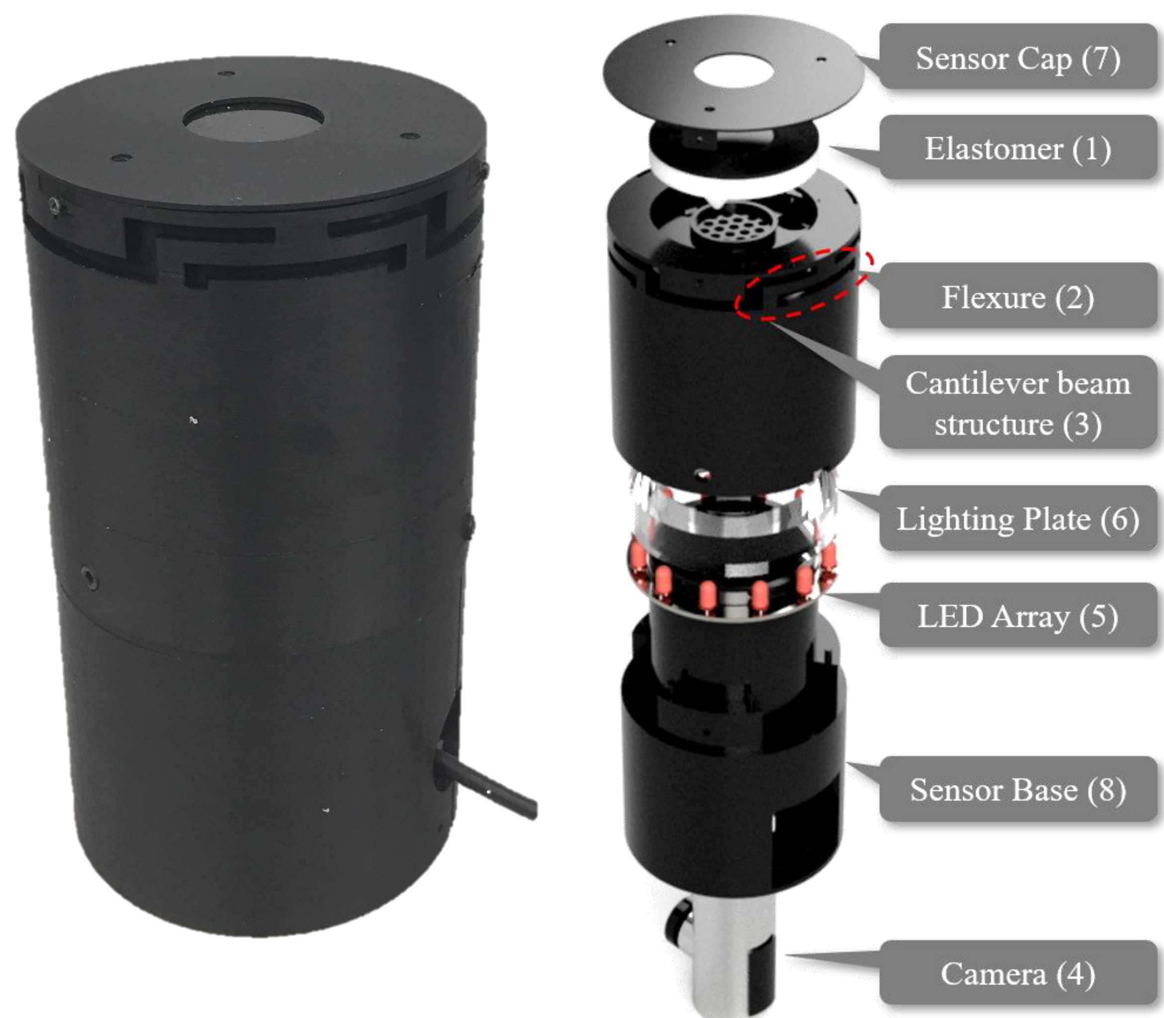
Fig.1 The design of the elastomer-based flexible optical force and tactile sensor. Left is the manufactured prototype, and right is the exploded view of the sensor structure.
